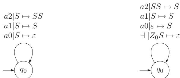
Fig. 7. Transition diagrams of the basic pushdown automata for ranked alphabet \mathcal{A} = \{a_2, a_1, a_0\} and trees in prefix (left) and postfix (right) notation from Example 4.3.
